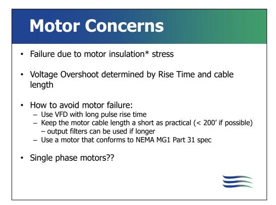
\*The motor's peak voltage rating doesn't correlate to the Insulation Class of the motor. The motor insulation class rating describes the temperature rating of the insulation and not its ability to withstand voltage peaks.
